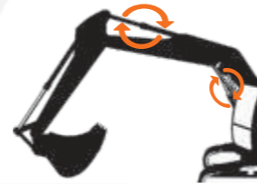
Boom & Arm Regeneration resulting in energy saving
